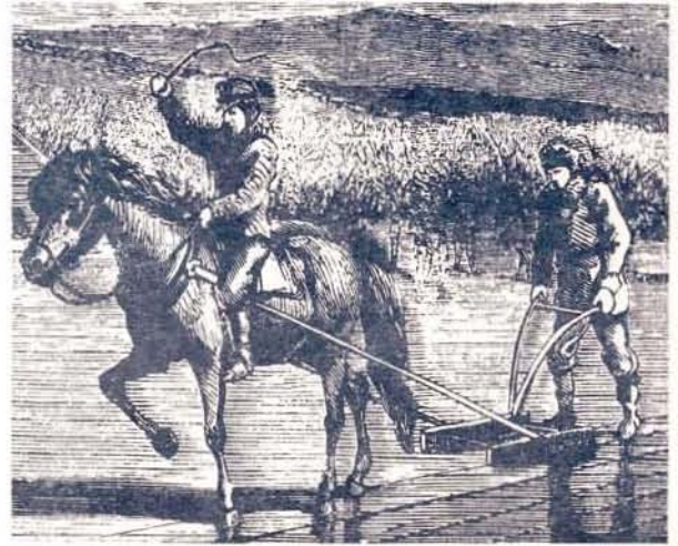
Marking the ice field with an ice plow.
